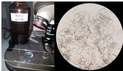
Figure 10. Crystallographic identification reaction of the SO 4 2- anion in the presence of barium chloride performed on a glass slide and evaluated with a Nikon E100 optical microscope (10x objective)
