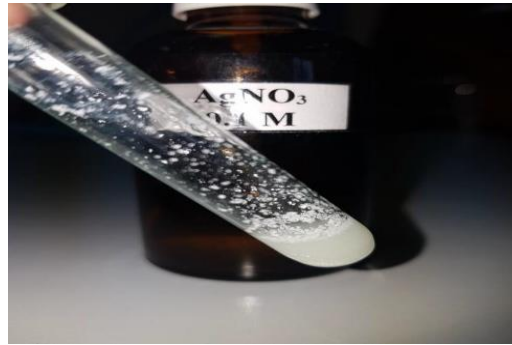
Figure 9. Identification reaction of the SO 3 2- anion in the presence of silver nitrate
