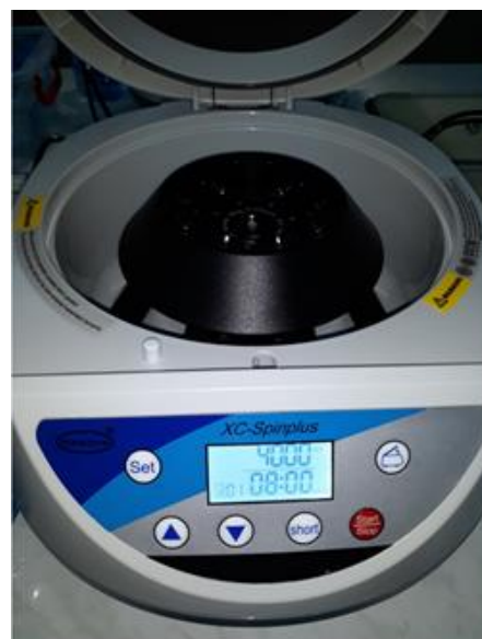
Figure 4. Programmable centrifuge, Rotor radius 100mm
