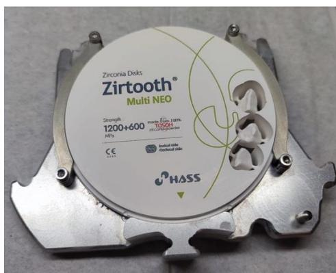
Figure 5. The milled zirconia elements
