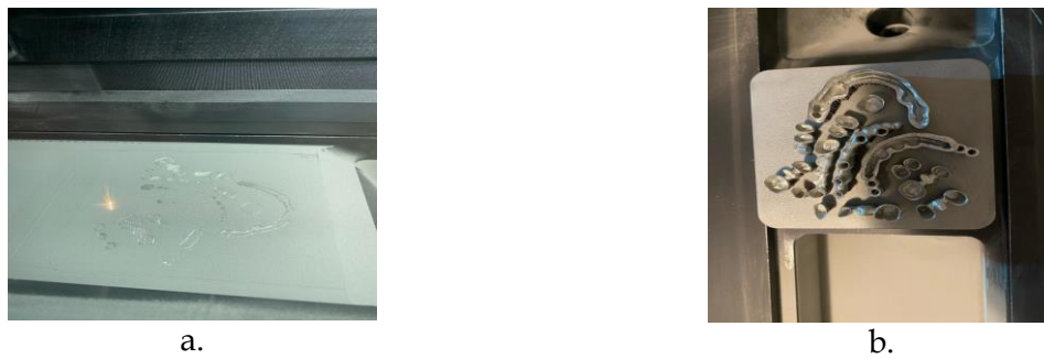
Figure 11. a. The powder bed; b. The actual laser sintering on the powder bed
