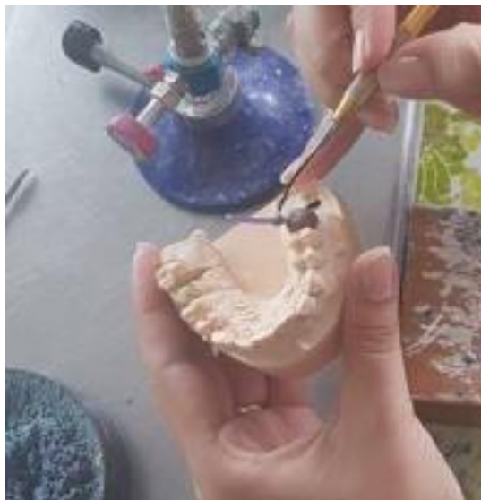
Figure 2. The sprue's attachment
