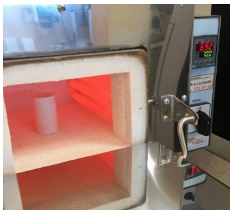
Figure 10. The preheating oven
