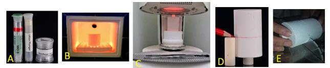
Figure 9. A. Ingots – IPS e.max Press – case 2; B. Preaheating oven – case 2; C. Ceramic furnace – case 2; D, E. Sectioning the mold – divesting procedure – case 2
