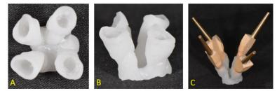
Figure 10. A, B. Pressed copings - case 1; C. Pressed copings adapted on the dies - case 1
