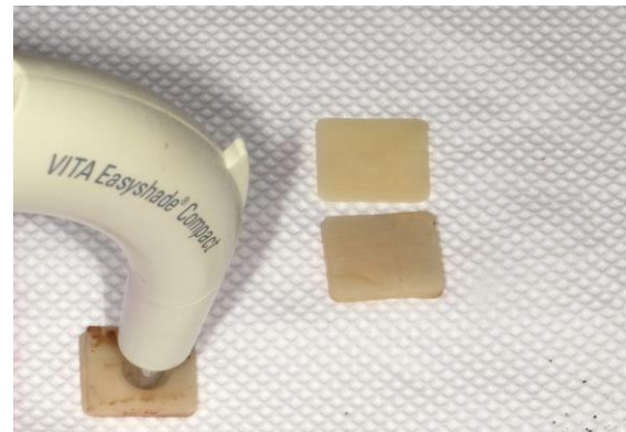
Figure 4. Spectrophotometric measurements with Vita Easy Shade after staining in vitro
