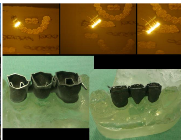
Figure 2. The metal infrastructures were produced using Phenix PXS Dental laser sintering machine from Phenix Systems (France)
