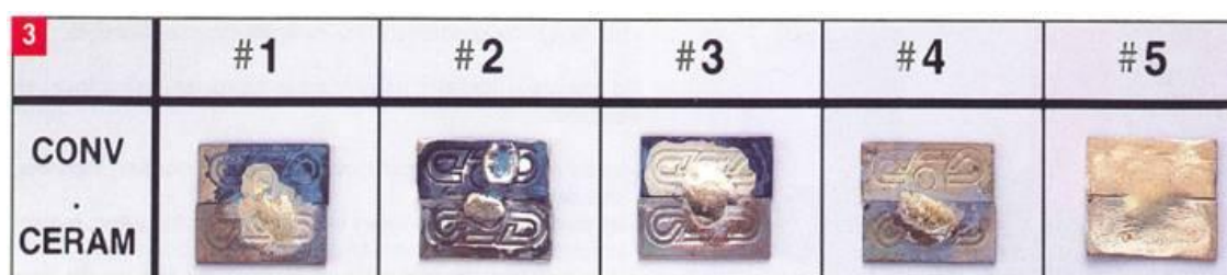
Fig. 3. Illustration of galvanic corrosion observed in the 5 samples (1-5).
