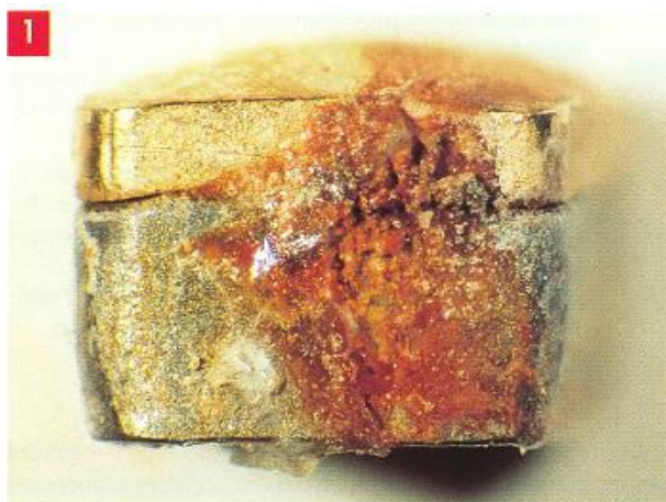
Fig. 1. Bimetallic wrist bracelet made of bimetallic rings gold/steel after corrosion in saline solution
