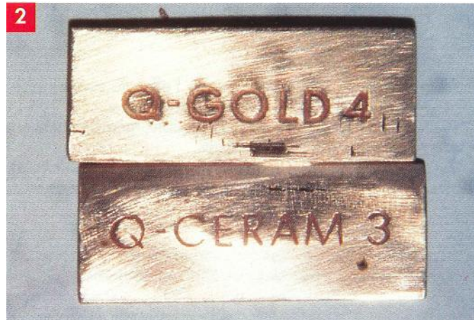
Fig. 2. The corrosion test samples are 2 plates of noble alloy connected by soldering
