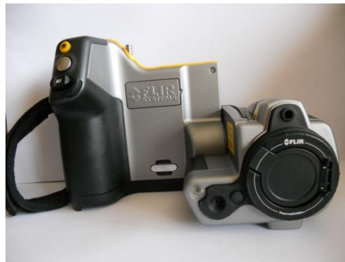
Fig.1 . The thermograph FLIR B200 (FLIR SYSTEMS, Hong Kong)
