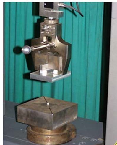
Fig.3 Zwick/Roel machine together with the specimen to be tested.
