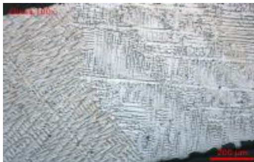
Fig. 12. Metallographic observation of a cast structure.
