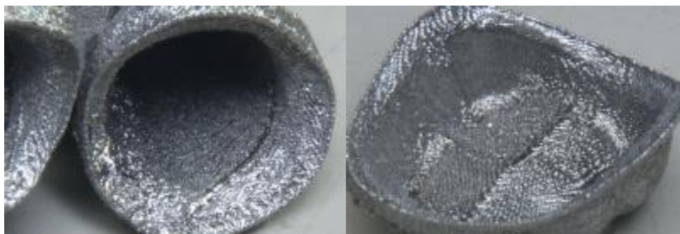
Fig. 8. The internal surface of two crowns, immediately after sintering.
