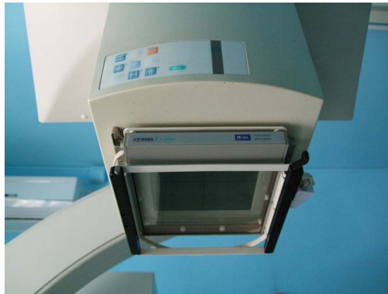
Fig.1 Removable DAP-meter mounted in front of collimator.
